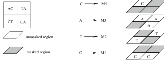
Fig. 1. Asynchronous synthesis of a 2 \times 2 microarray. The deposition sequence \mathcal{D} = \text{CTAC} corresponds to four masks \mathcal{M}_1, \mathcal{M}_2, \mathcal{M}_3, and \mathcal{M}_4 . The masked regions are shaded and the border between the masked and unmasked regions is represented by bold lines.
