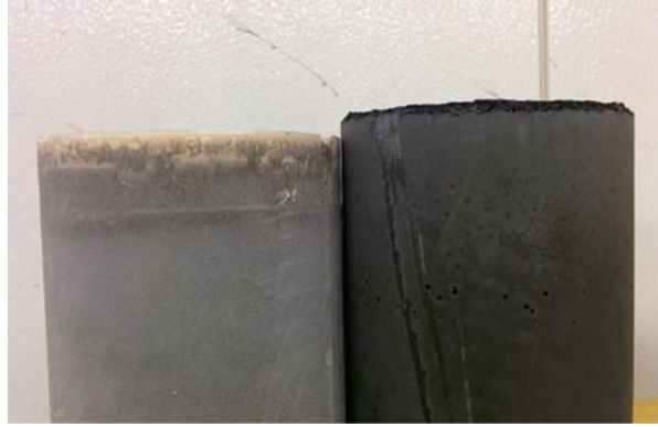
Fig. 4 Cylinders of plain paste ( left ) and CNF paste ( right ) after demolding
