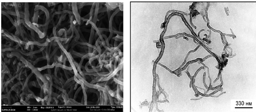
Fig. 1 The SEM image (left) and TEM (right) of functionalized CNTs
