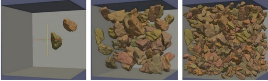
Fig. 1 Packing star shaped particles to model material mesostructure of mortar or concrete
