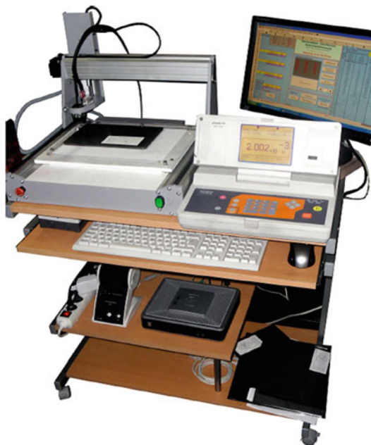
Fig. 19.6 Testing device for in-plane electrical conductivity measurement at Eisenhuth
