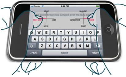
Fig. 3. Two-handed Marking Menus [17] employ multi-touch to draw parts of the Marking Menu strokes using alternating fingers.
