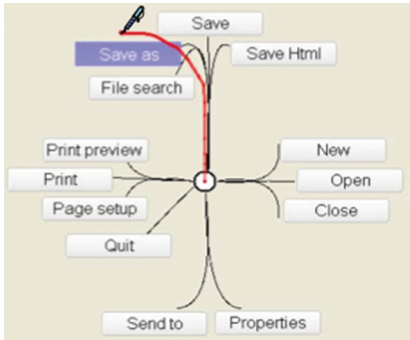
Fig. 5. The design of Flower Menus [2]. Each basic stroke direction (Up, Down, Left, Right) has 3 variations (straight, curved left/right).
