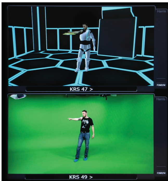
Fig. 1. The cyborg was created by partly overlaying the real, tracked actor with computer generated graphics within the green box.
