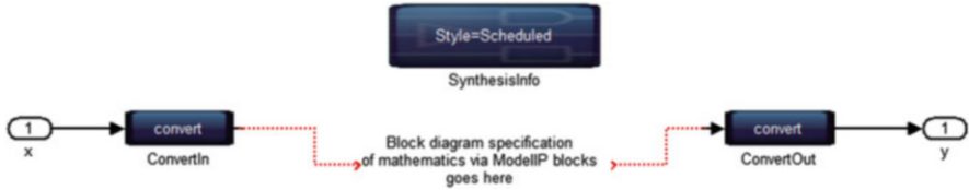
Fig. 9.14 We need a SynthesisInfo block for controlling synthesis flow. By using the default option of scheduled, we let DSP builder use a pipelining and delay distribution algorithm that create fast hardware implementations from an easily described untimed block diagram
