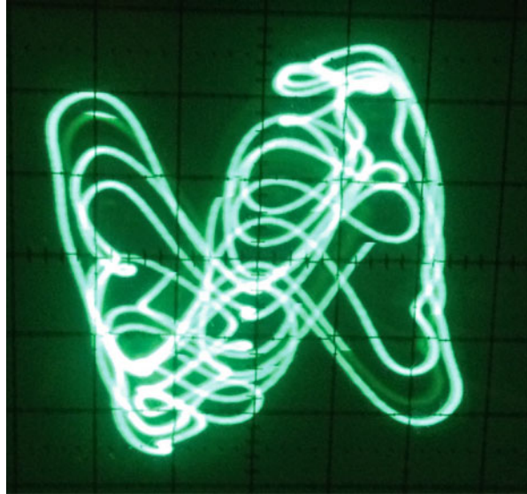
Fig. 9.17 x(t - \tau) vs. x(t) for the Ikeda DDE in Eq. (9.11). Oscilloscope scales are 0.5 V/div for both axis
