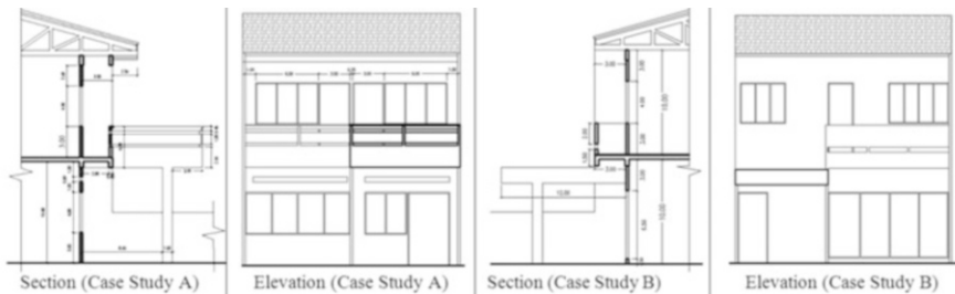
Fig. 25.2 Section and elevation in the Case Study A and B of the modern terraced house facade
