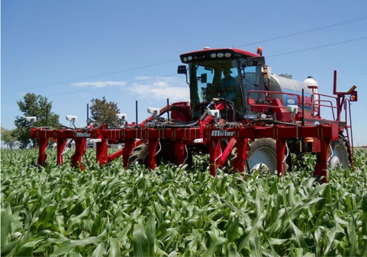
Fig. 2.7 A photo taken for sensor-based variable N rate application in a commercial corn field (Paul Raymer, The Farm Office in Ontario): Reflectance sensors are mounted in the front of tractor and instant collection of canopy N status data is used with a computer to determine the amount of N fertilizer needed for the specific locations. With variable rate controlled pump, precision N fertilizer is delivered to the specific locations in the field. How does this work? At planting, an N-rich strip ( \sim 200 \text{ kg ha}^{-1} ) is created for comparison, and rest of the field receives the regular start-up fertilizer. At sidedress stage, N-rich strip is mapped first and the resulting NDVI is used to adjust the algorithm for each field. Algorithm, programmed into the on-board computer, is used to control the variable rate of fertilizer application according to the plants requirement
