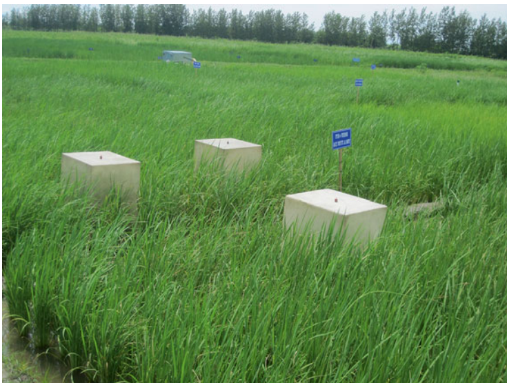
Fig. 5.1 Measurement of greenhouse gas emissions by closed chamber method in a paddy field in India
