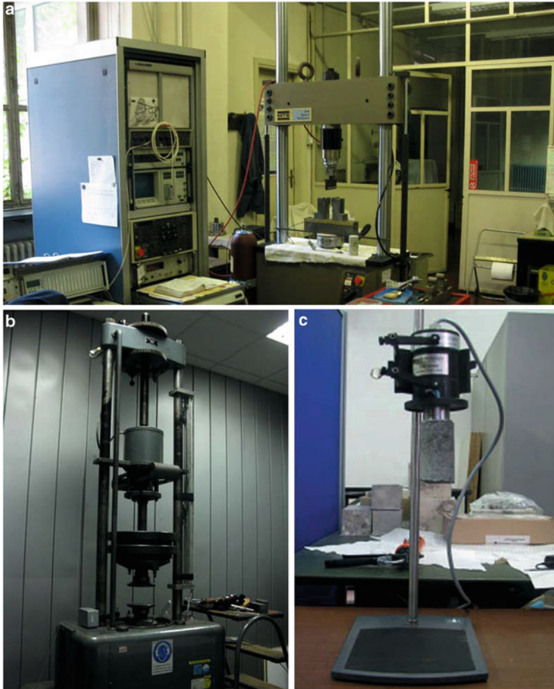
Fig. 4.2 Servo-hydraulic press employed during the low frequency fatigue tests (a) Electromechanical Amsler Vibrofore 10 HPF 422 used during the experimental test characterized by a frequency working range between 100 and 260 Hz (b). Bandelin HD 2200 sonotrode used during ultrasonic tests (c)
