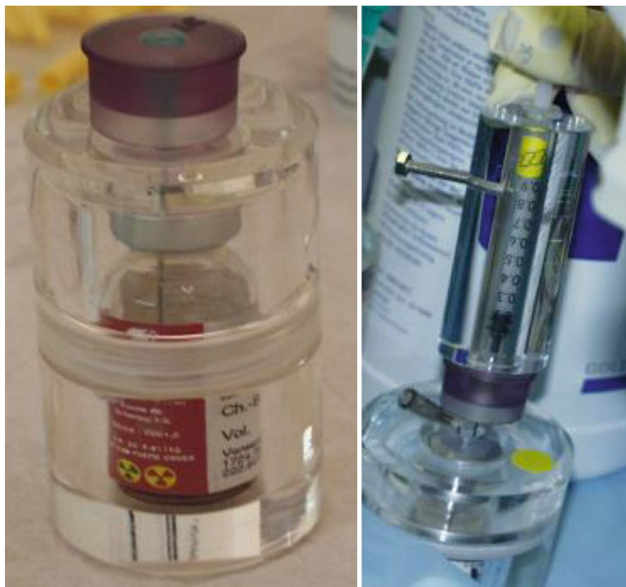
Fig. 8.3 Use of a Macrolonring™ during withdrawal of the syringes
