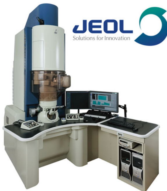
Fig. 1 JEM-ARM200F equipped with Cold Field Emission Gun
