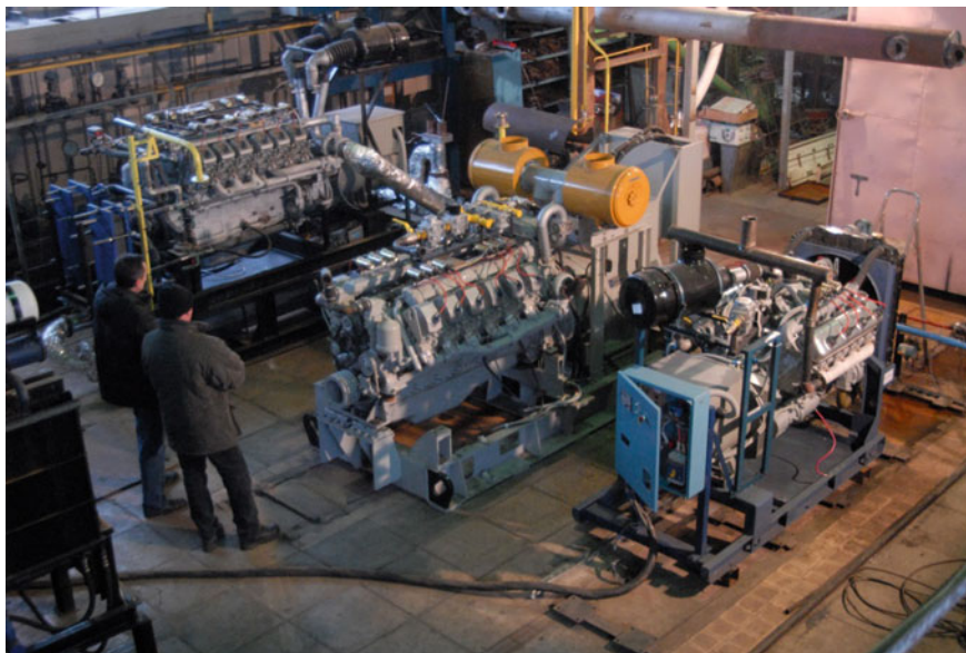
Fig. 1 General view of JIHT PAS experimental complex for working out regime parameters of gas piston installations which use natural gas and thermal processing of biomass products as a fuel
