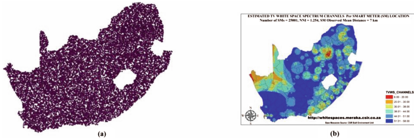
Fig. 3. (a) A spatial distribution of 25001 hypothetical smart meters in South Africa. The smart meters are assumed to be sending dynamic requests for white space spectrum resources from the GLSD (b). Snapshot of estimated spatially available spectrum resources returned as a response from the GLSD to the requesting smart meters. The dynamic interaction between smart meters and the GLSD is performed through PAWS service API.
