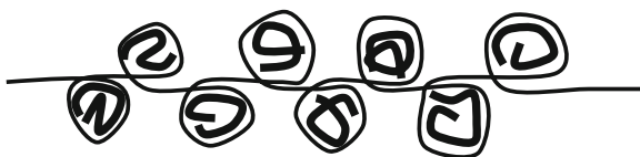
Scheme 8.3 Schematic structure of PEDOT:PSS in water. The thin and thick curves represent the PSS and PEDOT chains, respectively. Reproduced from [72]
