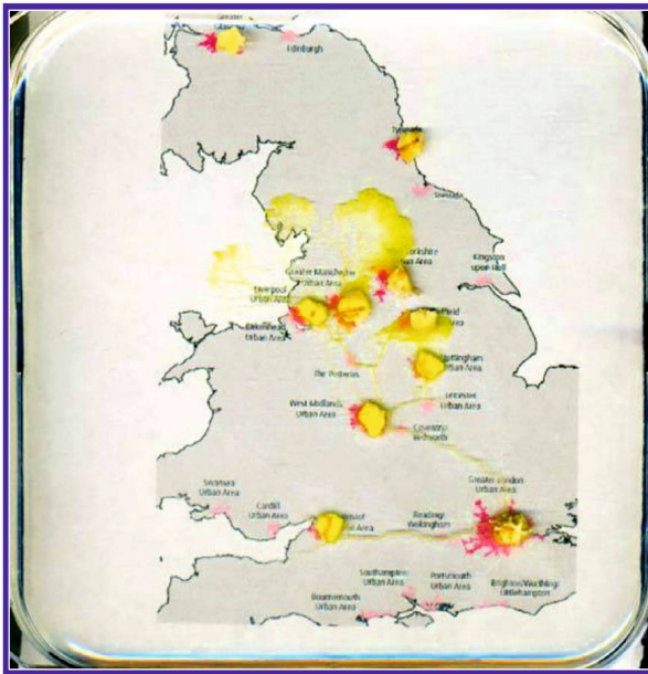
Fig. 2 The developing Physarum network adopted by [5]. Typical experimental setup of UK transportation network where ten most populous urban areas are represented by oat flakes, plasmodium is inoculated in London, the plasmodium spans oat flakes by protoplasmic transport network.
