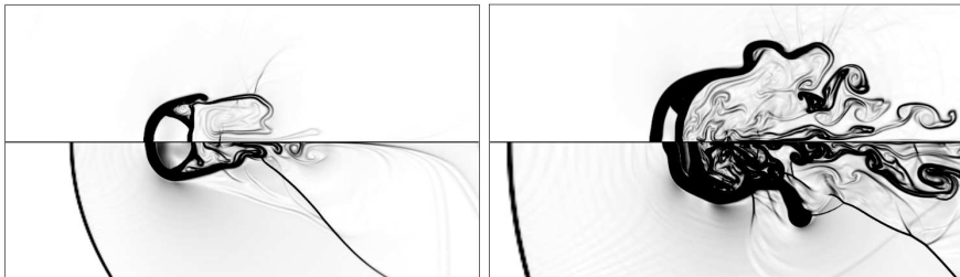
Fig. 3 Numerical schlieren images of the breakup behind Mach 1.47 ( top ) and Mach 2.50 ( bottom ) shockwaves at a t^* = 6.213 b t^* = 15.533
