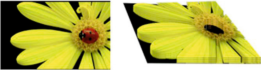
Fig. 16 Linguistic constraints derived by decision making system from meaningfulness cues. On the left is the original image. [29] On the right is spatial-taxon membership (height) inferred by autonomous decision making system. The x-y plane of the image is shown in skew. Height, fuzzy membership, is vertical. Note that both the black background and ladybug are at zero or close-to-zero membership. The system grouped the ladybug with the background, incorrectly inferring a hole in the flower.
