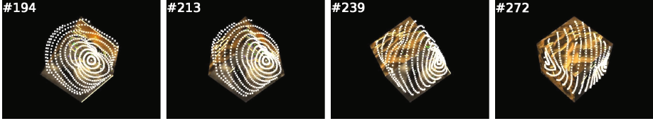
Fig. 5. Selected frames from the CUBE1 sequence. Notice, how TMAGIC learns the new face of the cube. #194: unknown shape, the surface is smoothed over. #213: first features detected, shape roughly estimated. #239: more features identified, shape refined. #272: Final state, model in agreement with the object.
