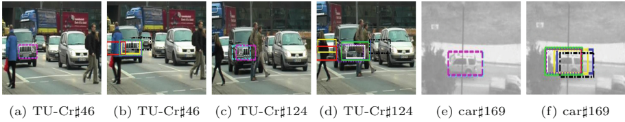
Fig. 4. Tracking through multiple partial occlusions. MTS-TS(magenta), MTS-L (cyan), SCM(green) FragT(white), Semi(yellow), L1-APG(blue), VTD(red), WLMCMC (black), and ASLA(purple) (Color figure online).
