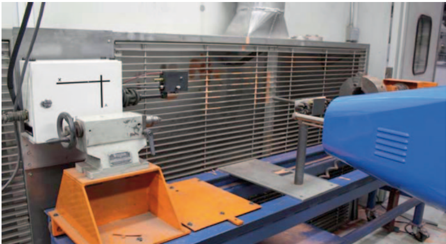
Fig. 8.12 The TECNAR ColdSprayMeter sensor head and scanner in action. (Courtesy of National Research Council of Canada)
