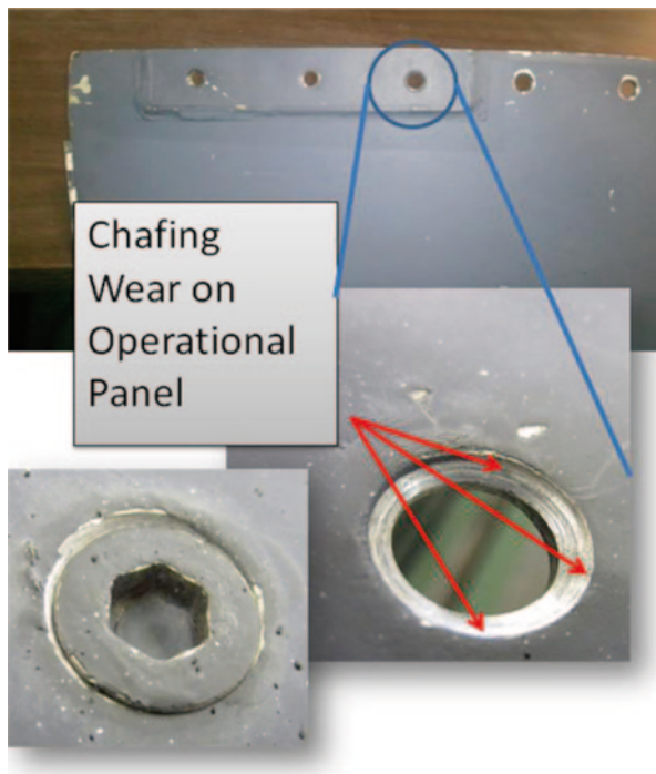
Fig. 10.8 Wear sites under fastener heads on FEB panels
