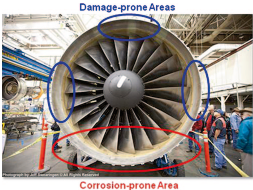
Fig. 10.17 Area on gas turbine engine fan case which is prone to corrosion due to retention of water
