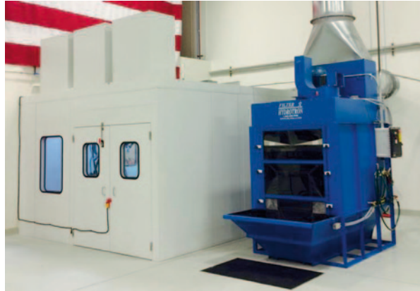
Fig. 6.18 Example of a fully enclosed acoustic spray booth for robotic cold spraying. (Courtesy of Able Engineering)
