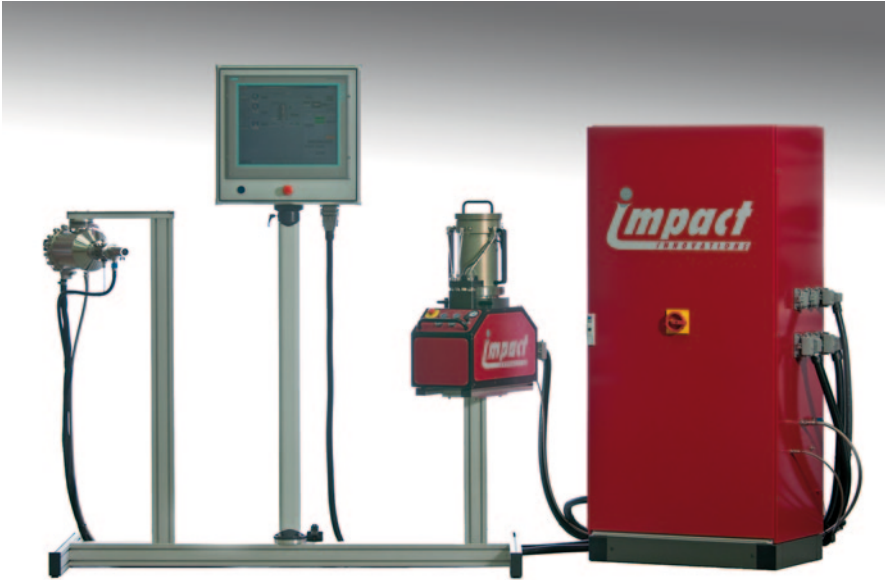
Fig. 6.7 Upstream injection cold spray system (40 kW/50 bar/1100°C) showing control unit, powder feeder, and water-cooled spray gun with a 40-kW gun-mounted gas heater. (Photo courtesy of Impact Innovations 2014)
