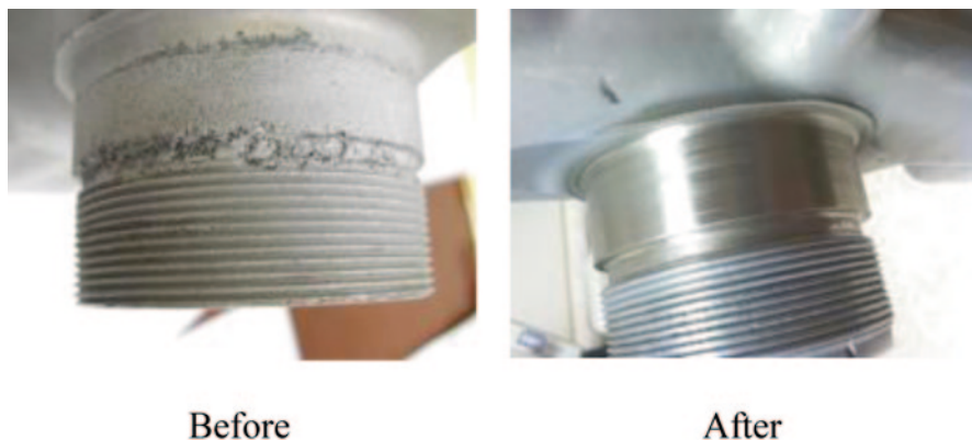
Fig. 10.21 Before and after photos of cold-sprayed repaired B737 nosewheel steering actuator barrel. (MOOG Aircraft Group 2012)
