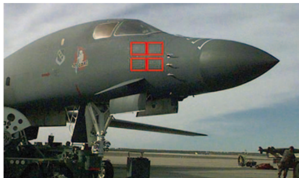
Fig. 10.7 FEB panels on B-1. There are eight panels per aircraft, four panels per left and right sides
