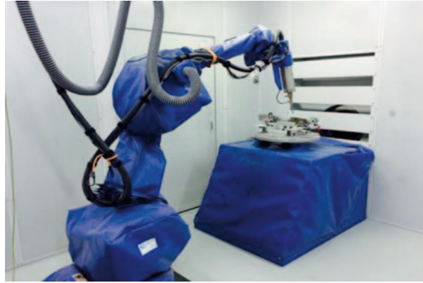
Fig. 6.12 Cold spray gun mounted on a multi-axis manipulator with the substrate or part mounted on a two-axis manipulator. (Courtesy of Able Engineering)
