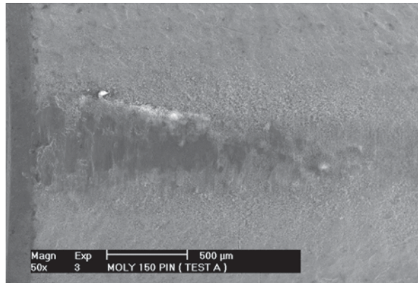
Fig. 10.33 Wear track of a cold-sprayed molybdenum coating after three million cycles of reciprocating wear. (Hager 2002)
