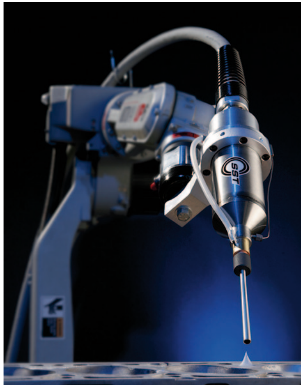
Fig. 6.11 Robotic cold spray gun mounted in a commercial multi-axis manipulator. (Courtesy of CenterLine (Windsor) Limited)
