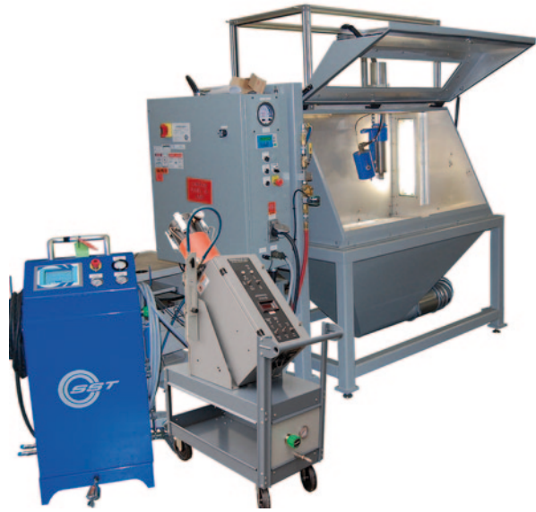
Fig. 6.4 Downstream injection system (15 kW/34 bar/550 °C) integrated with cabinet, ventilation, and auxiliary systems for mechanized operation. (Photos courtesy of CenterLine (Windsor) Limited)
