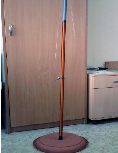
Fig. 1. Example of poorly constructed quarter-wave resonator coil
