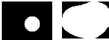
Fig. 3. Reference marker and detected object overlap test. Manually placed “reference” position marker on the left, segmented object mask on the right.
