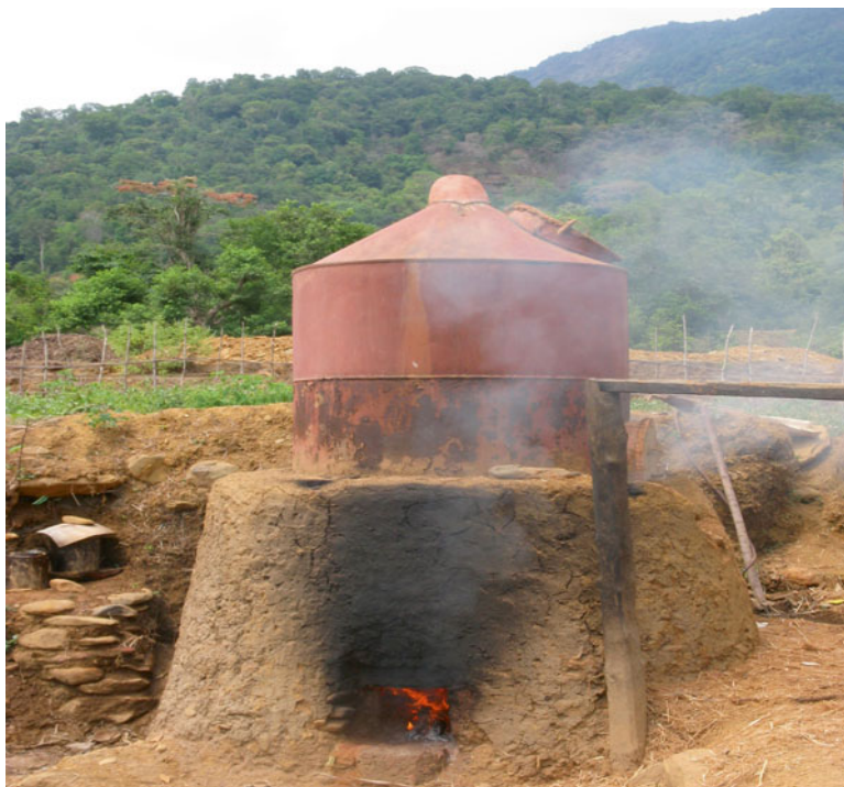
Fig. 10.5 Conventional distillation unit in a farmer's field in Western Ghats area, India. The traditional method of distillation of vetiver roots yield low essential oil yields, take more time and consume more fuel rendering the process less economical and environment friendly
