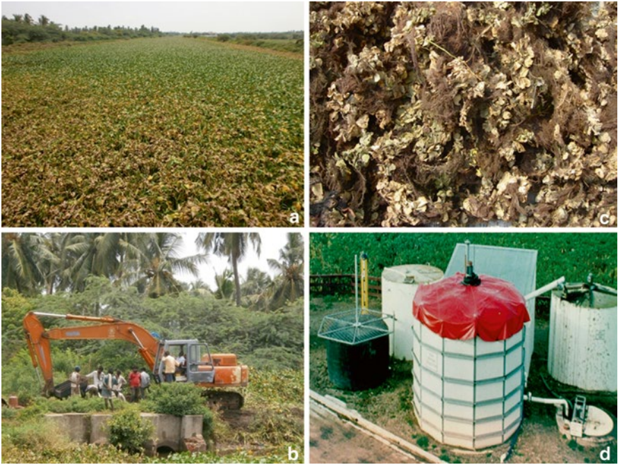
Fig. 7.44 (a–d) Harvested phytoremediated aquatic weed biomass is used as feed stock for biogas in anaerobic digester
