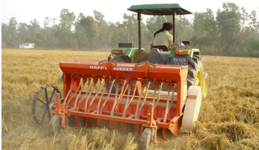
Fig. 3.3 Zero till sowing of wheat by happy seed drill in farmer field in (Punjab, India)
