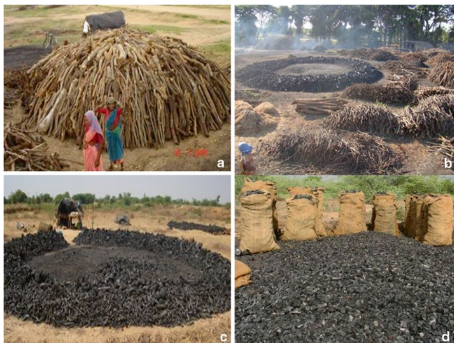
Fig. 7.29 Prosopis juliflora – charcoal production (a) Prosopis wood (b) Controlled burning to produce charcoal (c and d) Charcoal
