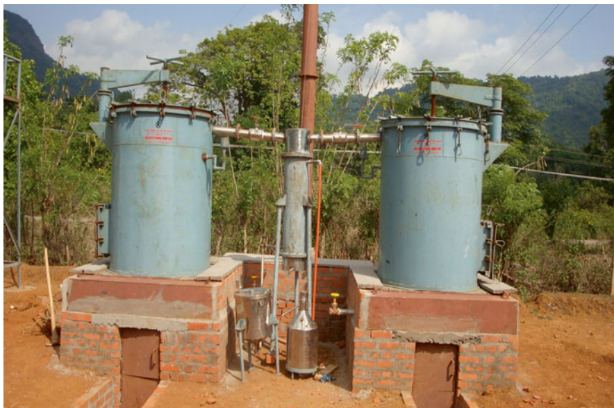
Fig. 10.6 Improved distillation unit and oil separator established in a farmer's field in Western Ghats area, India. The unit helps to recover more vetiver oil, consume less time and fuel making the process more economical and environment friendly
