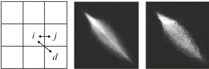
Fig. 44.2 Modified co-occurrence matrix. Left: Computing modified co-occurrence matrix. Center: Original co-occurrence matrix in normalized logarithm scale. Right: Modified co-occurrence matrix in normalized logarithm scale [FrEtAl11].
