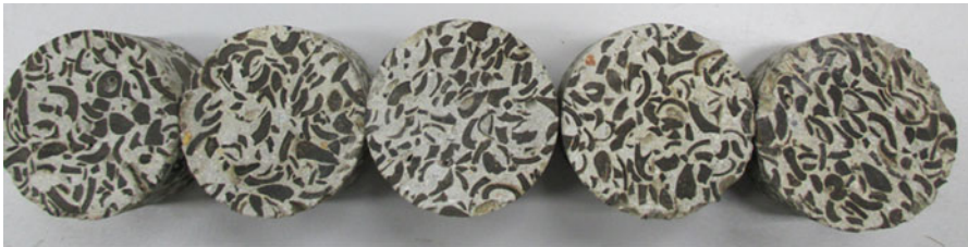
Fig. 30.4 Distribution of OPS in concrete (volume fraction from left: 30, 32, 34, 36 and 38 %)
