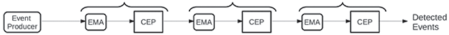
Fig. 10.3 Semantic enrichment of event streams. EMA event mapping agents, CEP complex event processing
