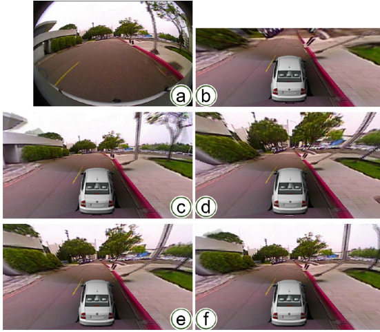
Fig. 14. The results using different 3D models. (a) Acquired image from fisheye camera. (b) After homography transformation. (c) Use ground plane and cylinder model. (d) Use second degree paraboloid. (e) Use fourth degree paraboloid. (f) Use hybrid model.
