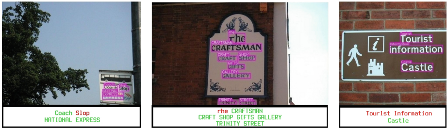
Fig. 4. Common misspelling mistakes using the CSER+Tesseract pipeline are due to missed diacritics, rare font types, and/or poor segmentation of some characters.
