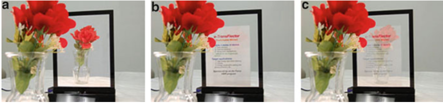
Fig. 7 Electrically switchable mirror based on a polymer stabilized cholesteric LC with a pitch gradient. (a) In reflection state; (b) In transparent state; (c) In half-reflection/transmission state. Courtesy: Kent Optronics
