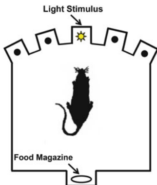
Fig. 1 Diagram of the five-choice serial reaction time task (5-CSRTT). In the 5-CSRTT, subjects are required to scan five apertures in an operant chamber for the appearance of a brief light stimulus (presented pseudorandomly) and to make a nose-poke response in the correct spatial location (i.e., the aperture where the light stimulus was presented) in order to receive a food reward
