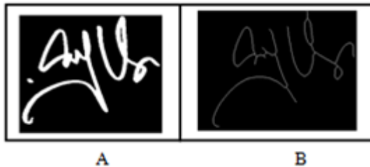
Fig. 6. A) Median Filter B) Ridge Thinning
