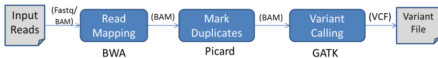
Fig. 1. The variant analysis workflow: The tools BWA, Picard, GATK are usually used for the three steps of the workflow. On the arrows, we write the different file formats of the processed data.
