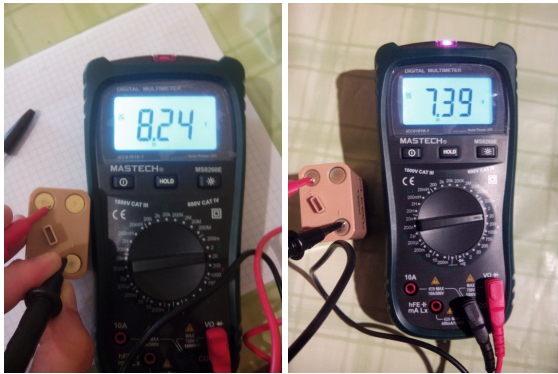
Fig. 5. In the first picture the battery works perfectly. Once Pleo has no power to make it run its battery have exactly 7,39V.
