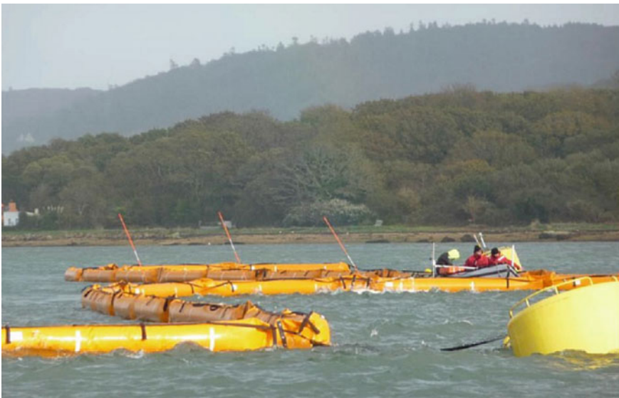
Fig. 7.9 Boom geometry measurement with GPS
