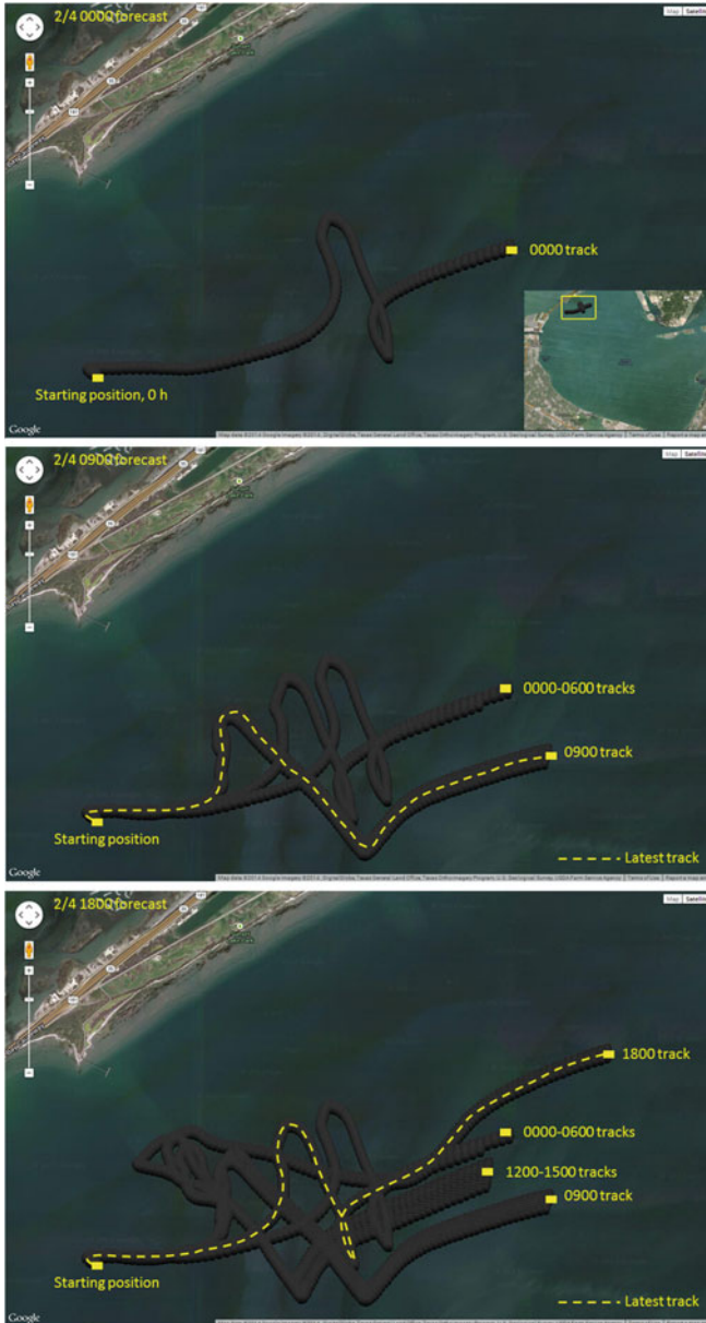
Fig. 5.5 HyposPy visualization of forecast tracks for an imaginary oil spill in Corpus Christi Bay (Texas, USA). Upper frame is the initial forecast track available within minutes of the spill. The middle frame is the forecast tracks available at 0900 using new wind forecast data. Note the 0000–0600 forecasts are almost indistinguishable in their prediction of the 48 h position. Lower frame shows predictions in the afternoon initially move away from and then back toward the beach. Continued in Fig. 5.6. Visualization using Google Earth with additional annotations (in yellow) for clarity
