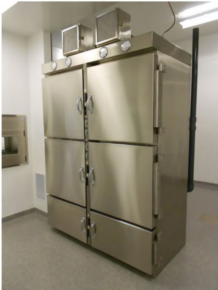
Fig. 7.4 Four commercial minicells, inside each of which a synthesis box for synthesis of PET radiopharmaceuticals is installed (picture provided by Radiation Shielding, Inc.)
