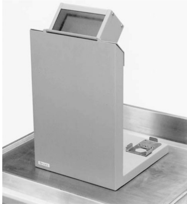
Fig. 10.4 Lead barrier shield (L-block), behind which all formulation and handling of radioactive materials are carried out (Photo courtesy of Biodex Medical Systems Inc., NY)
