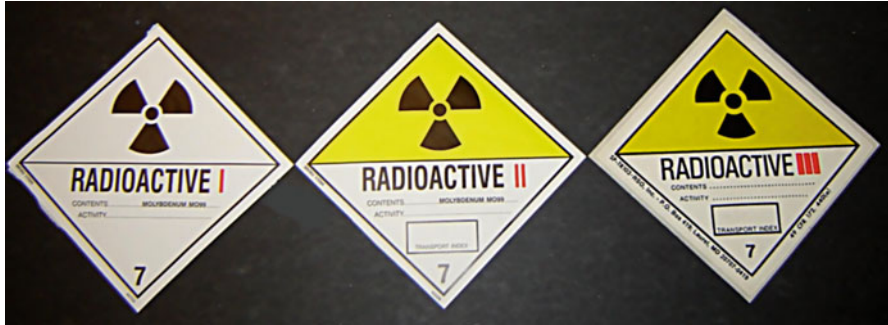
Fig. 10.6 Three types of US DOT labels required for transportation of radioactive materials. (Fig. 16.3 on p 329, Radiation Regulations and Protection , in: Gopal B Saha (2013), Physics and Radiobiology of Nuclear Medicine , Springer; With kind permission from Springer Science and Business Media)
