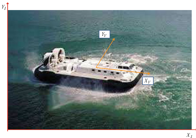
Fig. 6.76 Underactuated hovercraft performing maneuvers and the associated reference frames
