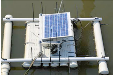
Large observation buoy with YSI instrumentation and telemetry
