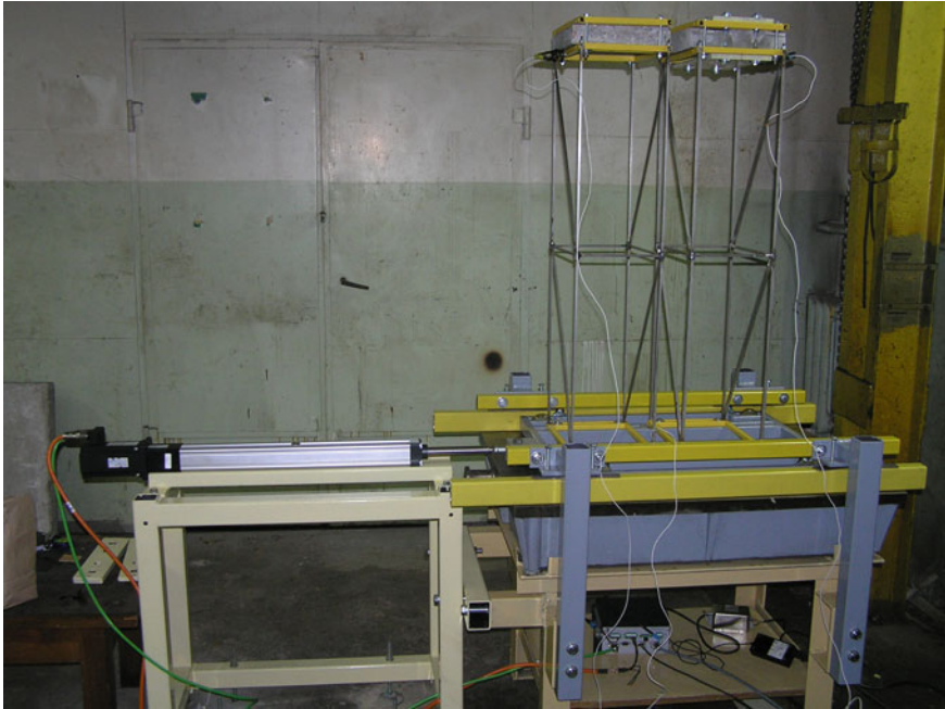
Fig. 2.10 Setup of the shaking table experiment
