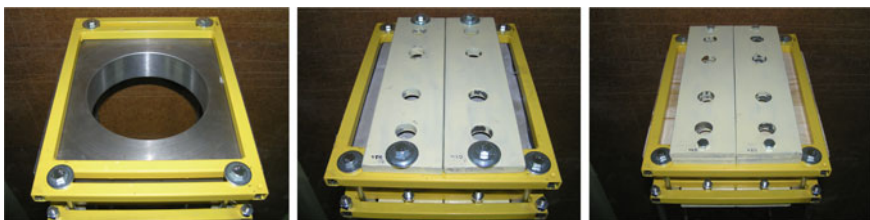
Fig. 2.12 Top view of the right tower with impacting elements (made of steel, concrete and timber) and additional masses
