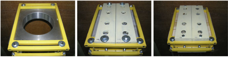
Fig. 2.12 Top view of the right tower with impacting elements (made of steel, concrete and timber) and additional masses
