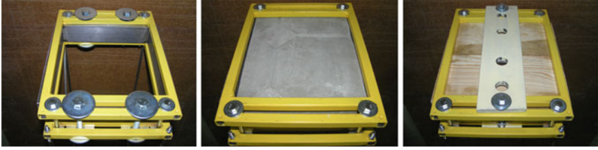
Fig. 2.11 Top view of the left tower with impacting elements (made of steel, concrete and timber) and additional masses
