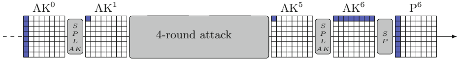
Fig. 9. The 4-round attack is extended by one round in the beginning and one round in the end to mount an attack on 6.5 rounds.
