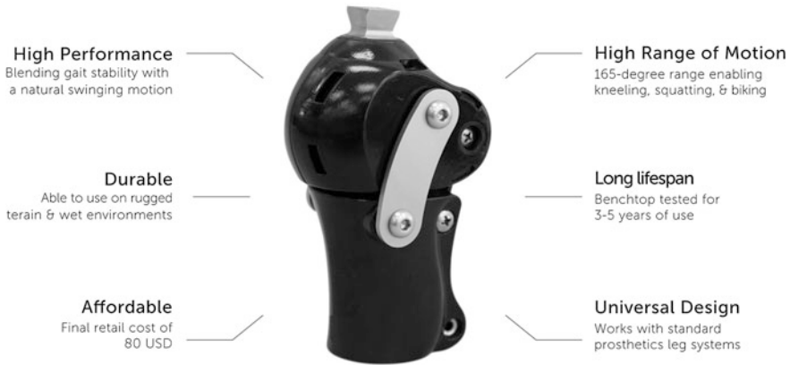
Fig. 14.5 A ReMotion Knee prototype. These prototypes were assembled in California for field testing at clinics in India, Indonesia, and Guatemala. Added features included curvature mimicking anatomical knee cap, noise dampening, and standardized attachment systems (i.e., pyramid and 30 mm pylon). The latest version of the ReMotion Knee will be available for clinics to purchase in the second quarter of 2015
