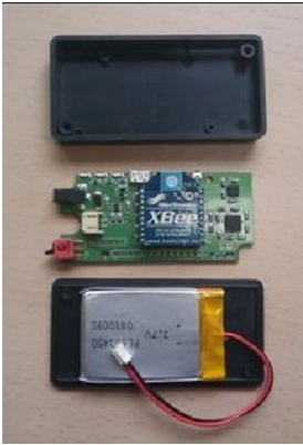
Fig. 8. WAGYRO energy harvesting device [26]
