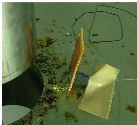
Fig. 5. Gamma radiation experiment of a laser (VCSEL-AS-0001-K: Fuji Xerox Co. Ltd.). The wavelength is 850 nm. The VCSEL was exposed up to 10 Mrad cobalt 60 gamma radiation. Even after a VCSEL was exposed to 10 Mrad radiation, the VCSEL functioned correctly. No degradation of the voltage current relation and light power was found.
