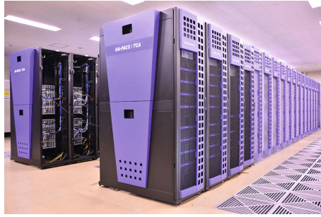
Fig. 2. Photograph of the Entire HA-PACS System (HA-PACS/TCA: 5 racks × 2 rows, HA-PACS base cluster: other racks)
