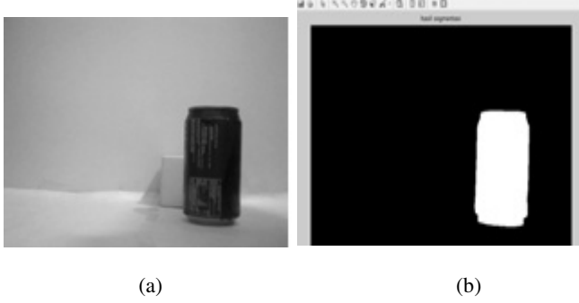
Fig. 1. (a) Original image contained a can as an object of interest and a yellow box as an object background (b) A can was separated from the background after segmentation process using region growing approach
