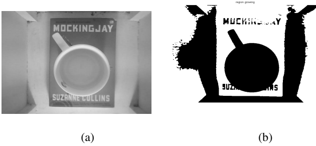
Fig. 2. (a) Original image before segmentation (b) Image segmentation result using region growing
