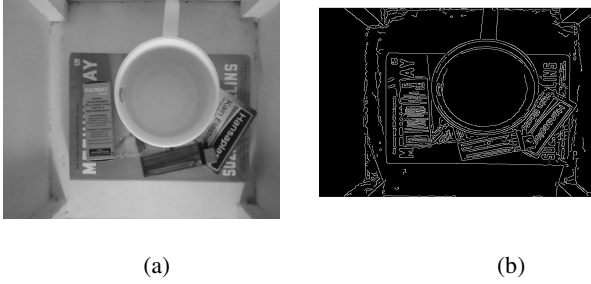
Fig. 6. (a) Original image before segmentation (b) Image segmentation result canny edge
