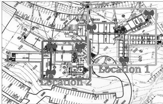
Fig. 2. Experiment Location (Location 1, Location 2). The icon of wireless transmitter refers to the location of the WLAN access point which is attached with the FM local transmitter.
