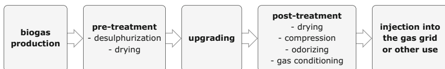
Fig. 8.7 Schematic diagram of the biogas upgrading process
