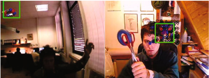
Fig. 2. Snapshots of the hand and torus sequences showing typical Matrioska failure cases: texture-less objects and non-rigid transformations
