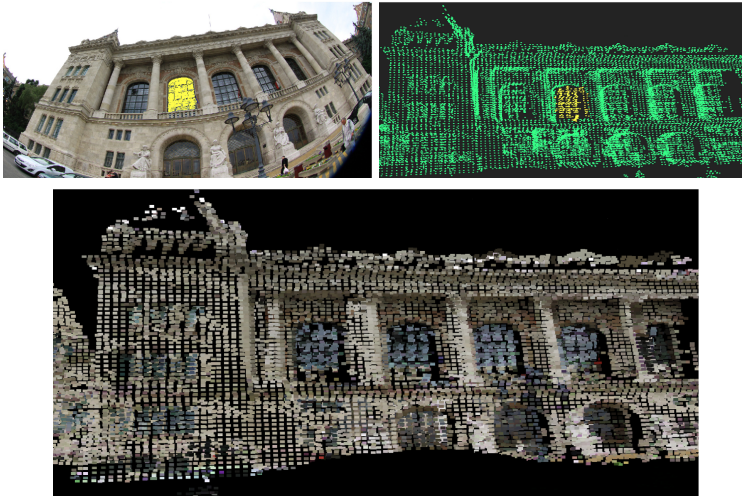
Fig. 7. Dioptric (fisheye) and lidar images with segmented area marked in yellow, and the fused images after pose estimation (best viewed in color)
