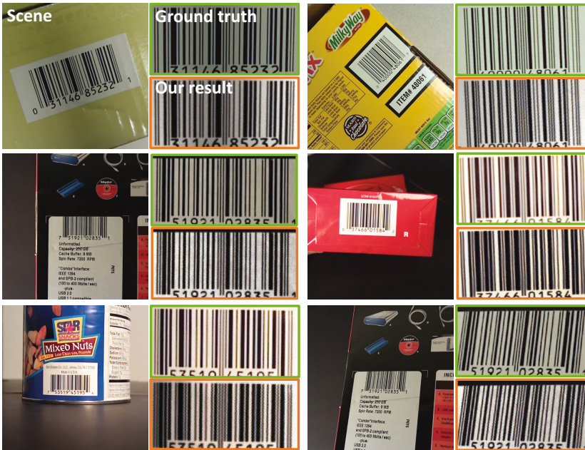
Fig. 9. Rendering results of real barcodes using our scanning system. The full image on the left of each barcode example is the in focus image at the ground truth depth. Our rendering results are shown with orange boundary, while the ground truth are shown with green boundary for comparison.
