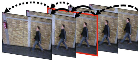
Fig. 4. Visualization of the Temporal MIP extension. Standard MIP encodes three successive frames, t - 1 , t and t + 1 (solid arrows). Temporal MIP additionally encodes frames t - 1 , t and t + 2 (dotted arrows), and frames t - 2 , t , and t + 1 (dashed arrows). Frame t is emphasized in red.
