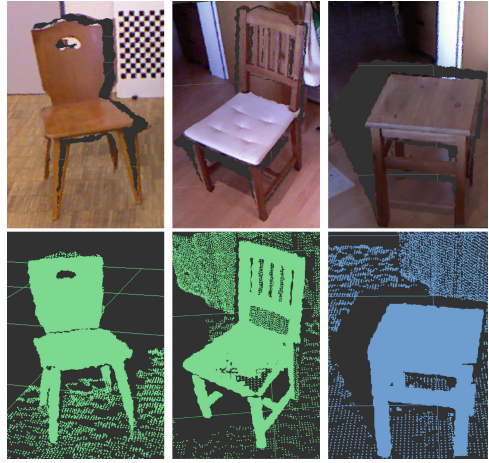
Fig. 2. The top row shows example objects from our evaluation. Chairs and stools served for the two fine-grained affordances. The bottom row presents affordance detection results: the sitting with backrest affordance is shown in green, whereas the sitting without backrest affordance is shown in blue.
