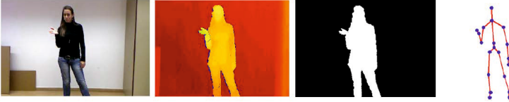
Fig. 1. An example from the dataset: RGB video, depth video, user mask video and skeleton data (left to right)
