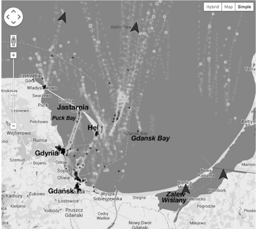
Fig. 14.2 A sub-pattern of traffic for course N, and examples of detections (potential violations)
