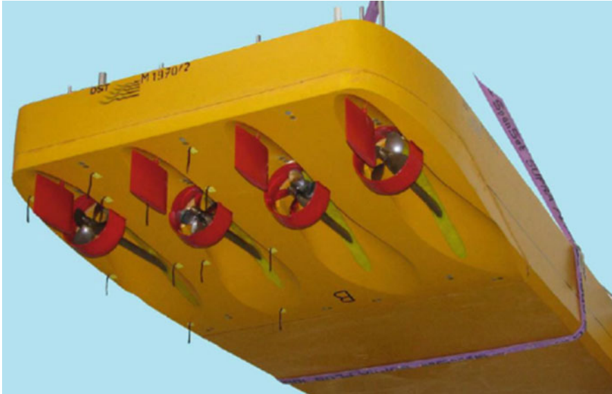
Fig. 20.8 Aft ship arrangement of alternative power configurations
